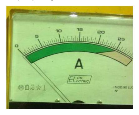
...If the pointer is more the 1 amps, decrease the position of the second and third knob regulation 'till the 0.5/1 amps setting is reached.
